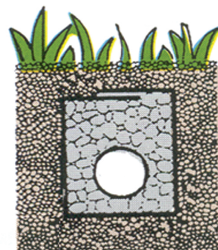
TerraTex® Nonwoven is commonly used as a liner in French drain trenches.
